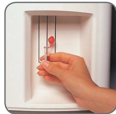
Step 2: Add EDTA sample and press start
